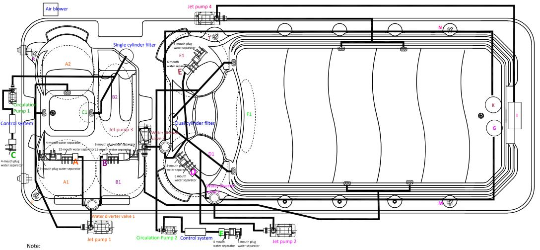
Jet pump 1 is connected to water diverter valve 1, which is connected to group A and group B water distributor. Group A water distributor is connected to the A1 and A2 jets, Group B water distributor is connected to the B1 and B2 jets.
